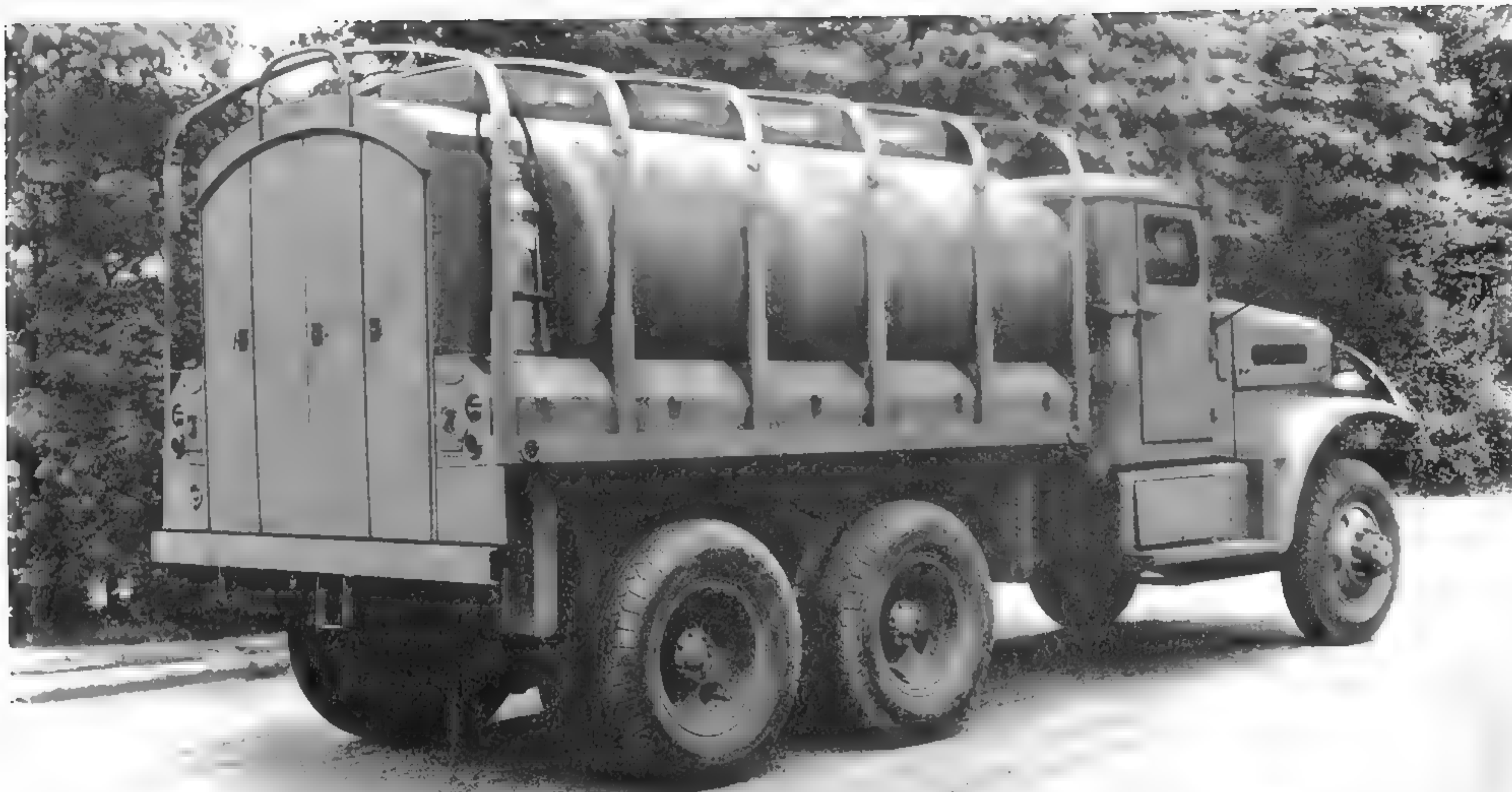
Only 25 of these huge 2,000-gallon fuel tankers were built by White, making them the scarcest of the 6-ton trucks. They featured self-sealing four-compartment tanks built by Butler. There were provisions to install bows and canvas to camouflage them as cargo trucks. (White Motor Company photo)
